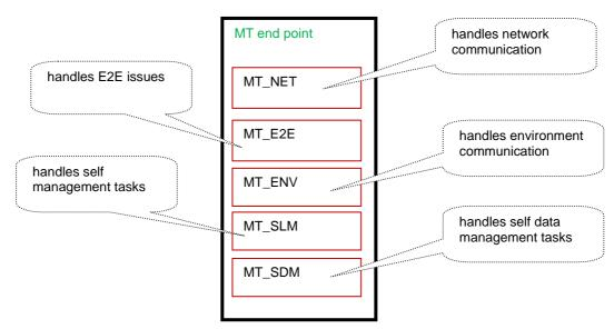
Figure 10: System endpoint components
