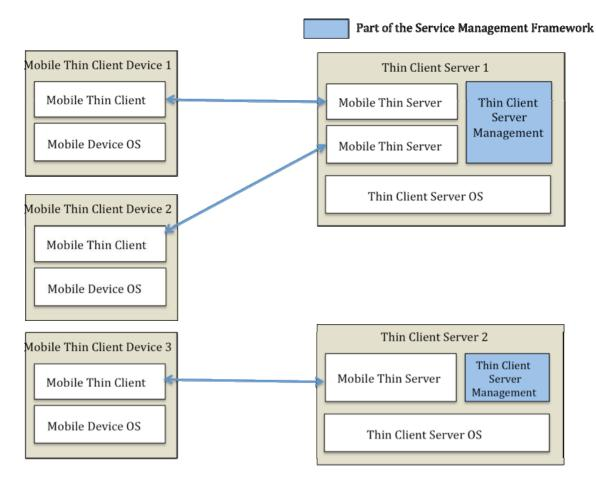
Figure 2: Multi-user aspect of the system Architecture
