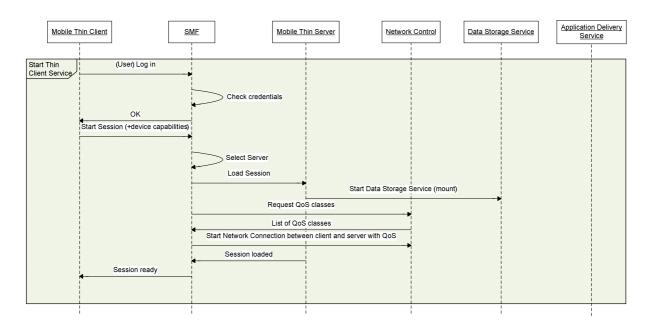
Figure A.1: Sequence diagram "Start the thin client service"
